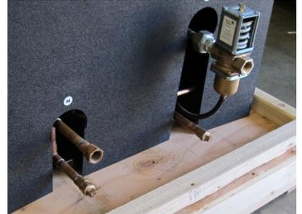
3. Connect the plumbing from the pool to the heat exchanger FPT PVC water fittings on the front of the chiller. Be careful not to over tighten the plastic fittings. See “Chiller By-pass Plumbing”
